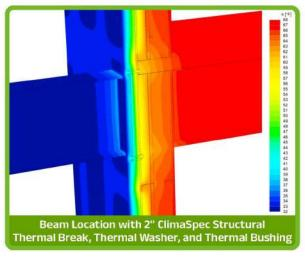
Increasing the thickness of the ClimaSpec TB Structural Thermal Break, using stainless steel bolts, while adding ClimaSpec Thermal Washers and Bushings significantly improves the energy performance of the connection due to the reduction in thermal transmittance (chi value). The table below provides several scenarios highlighting the increased energy efficiency when continuously improving the thermal design of the connection.
